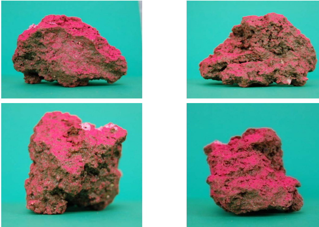
Figure 4. Views of a treated (large) clod after multiple applications of the tracer fluorescent dye.
